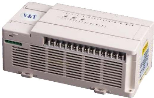
VC10V series is a simple motion control PLC, is a simple sport programmable logic controller with 4 pulse outputs based on the VC10 series, built-in 2-channel 100KHz + 2-channel 60KHz high-speed pulse outputs, 2-channel 50KHz high-speed counting. It has all the functions of VC10, and optimizes and improves the performance of VC10, making it extremely cost-effective.
